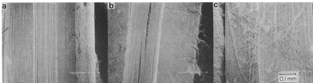
Figure 14 Scanning electron micrographs of the longitudinal section of POM tubes; draw ratios: (a) 10, (b) 21; (c) 33
